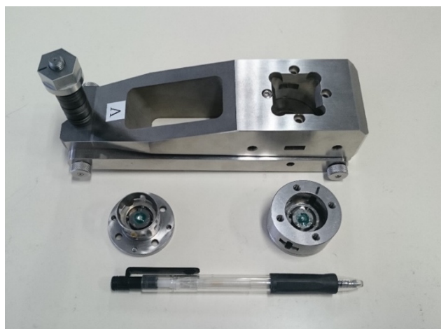
Fig.2 Photograph of lever-type diamond anvil cell (DAC) called "KUJIRA-type".
