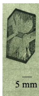
Fig.1 Domain patterns of as-grown TGS with positively charged carbon powder decoration method. Dark and light areas are negative and positive domains, respectively. 15)
