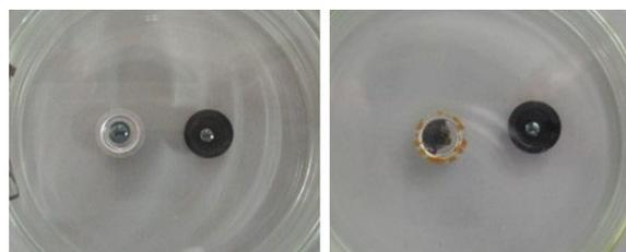
**Fig.7** Photos of DES containing iodine in a common aluminum pan (silver, left-hand side) and a fluororesin-coated aluminum pan (black, right-hand side). Photos on the left-hand side and the right-hand side are of just after putting and 14 hours later, respectively.
