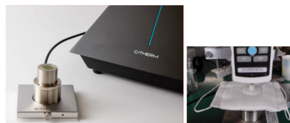
Fig.1 Modified Transient Plane Source (MTPS) of TRIDENT system, and compression test accessory (CTA).
