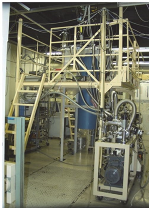
Fig.5 Constant volume gas thermometer. (Photo by AIST)
