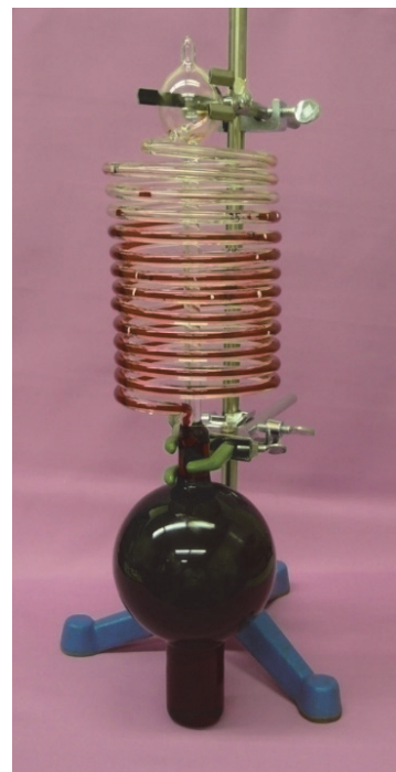
Fig.2 Liquid in glass thermometer from 17 th century Italy (Replica, owned by AIST) (Photo by AIST).
