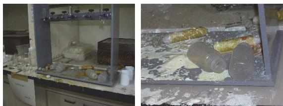
Fig.1 Explosion accident of ion exchange resin at Ningyo-toge Environmental Engineering Center of Japan Atomic Energy Agency (JAEA).
