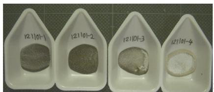
**Fig.13** Air drying experiment (#121101-1 ~ 4) aqueous ammonia (1 g) was mixed with  $\text{Ag}_2\text{O}$  of 38 mg (-1), 30 mg (-2), 20 mg (-3), 10 mg (-4).
