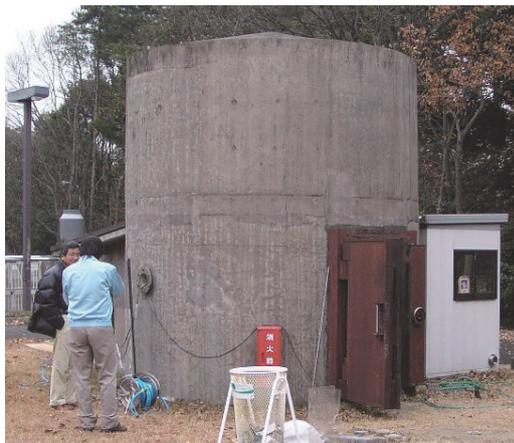
Fig.8 Explosion chamber for gram scale explosion test, inner diameter 2.9 m, height 3.45 m.
