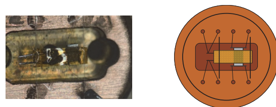
Fig.3 A photo picture and a schematic drawing of the thermal relaxation calorimetry cell of which sample stage is rigidly supported by thin stainless wires.
