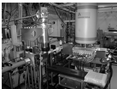
Fig.12 XAS system installed in BL14B2 at SPring-8. Measurement mode: transmission, fluorescence and conversion electron yield. Temperature and atmosphere: 4.2~1300 K, reduction ~ oxidation state and etc. This system possesses the automatically measurement equipment for high throughputs, and it is very easy to use this system for beginner. 29, 30)
