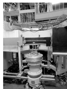
Fig.14 HRPD, i.e. neutron diffraction, system in JRR3 at JAEA. Measurements mode: transmission using vanadium folder. Temperature: 4.2~750 K, Wavelength: 1.16~2.97 Å. This system possesses high efficient detector system with 64 detectors.
