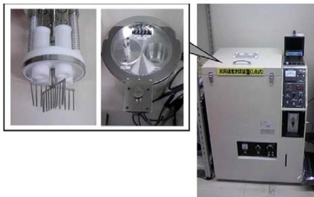
Fig.7 Measuring equipment for the hydration rate.
