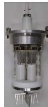
Fig.5 Mixing system of conduction calorimeter.
