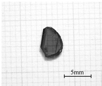
Fig.11 A photograph of a single crystal of SrIn<sub>2</sub>Se<sub>4</sub>.
