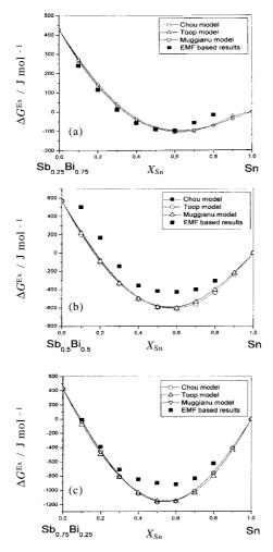
**Fig.2** Model calculation of excess free energy of mixing in the ternary alloys at 900 K by using reference data. (a) Sb<sub>0.25</sub>Bi<sub>0.75</sub>-Sn. (b) Sb<sub>0.50</sub>Bi<sub>0.50</sub>-Sn. (c) Sb<sub>0.75</sub>Bi<sub>0.25</sub>-S.
