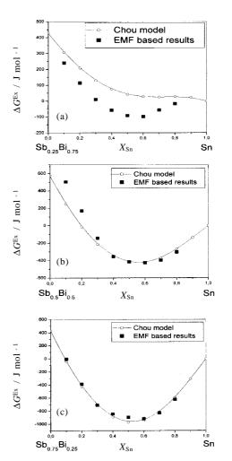
$\label{eq:Fig.3} \begin{array}{ll} \textbf{Fig.3} & \textbf{Model caluculation of the excess free energy} \\ & \textbf{of mixing in the ternary alloys at 900 K by} \\ & \textbf{using present data. (a)} & \textbf{Sb}_{0.25}\textbf{Bi}_{0.75}\textbf{-Sn. (b)} \\ & \textbf{Sb}_{0.50}\textbf{Bi}_{0.50}\textbf{-Sn. (c)} & \textbf{Sb}_{0.75}\textbf{Bi}_{0.25}\textbf{-Sn.} \end{array}$
