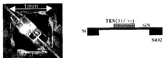
Fig.10 Schematic view and photographs of a calorimeter made on a SiN membrane. The TES is deposited on the SiN membrane of 1 μm thickness which has a bridge-like structure.
